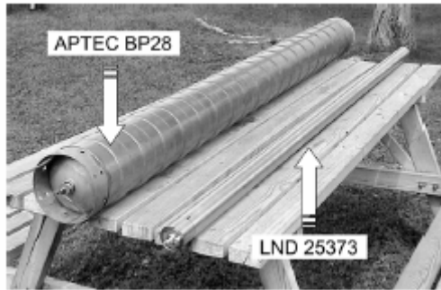
Fig. 1. Picture of the two proportional counters in use by the SVIRCO Observatory & TPL (Rome – Italy).
