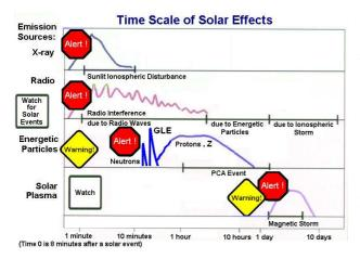
Fig. 1: Time scale of the response to solar disturbances at Earth and scale of prognosis by NOAA
