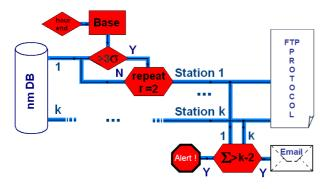
Fig. 4: Block-scheme of the system of generation of alert system for proton ground level enhancement
