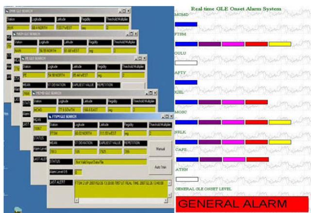
Fig. 3. The scripts that read data from NM stations (left panel) and the actual Alert signal displayed at the Athens NM station webpage (right panel).
