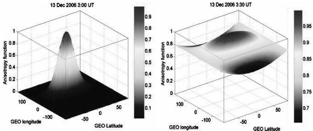
Fig. 5. Anisotropy function versus geographical latitude and geographical longitude of the anisotropy source, according to the NM-BANGLE Model. Left panel corresponds to 13 December 2006 at 3:00 UT, whereas the right panel at 3:30 UT.
