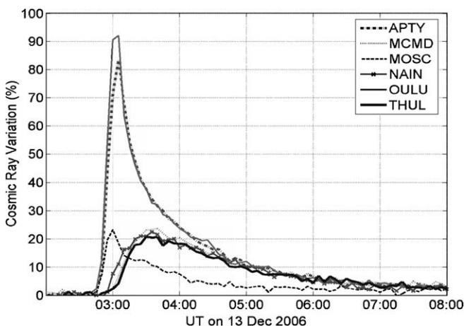
Fig. 1. GLE70 recorded by neutron monitors.
