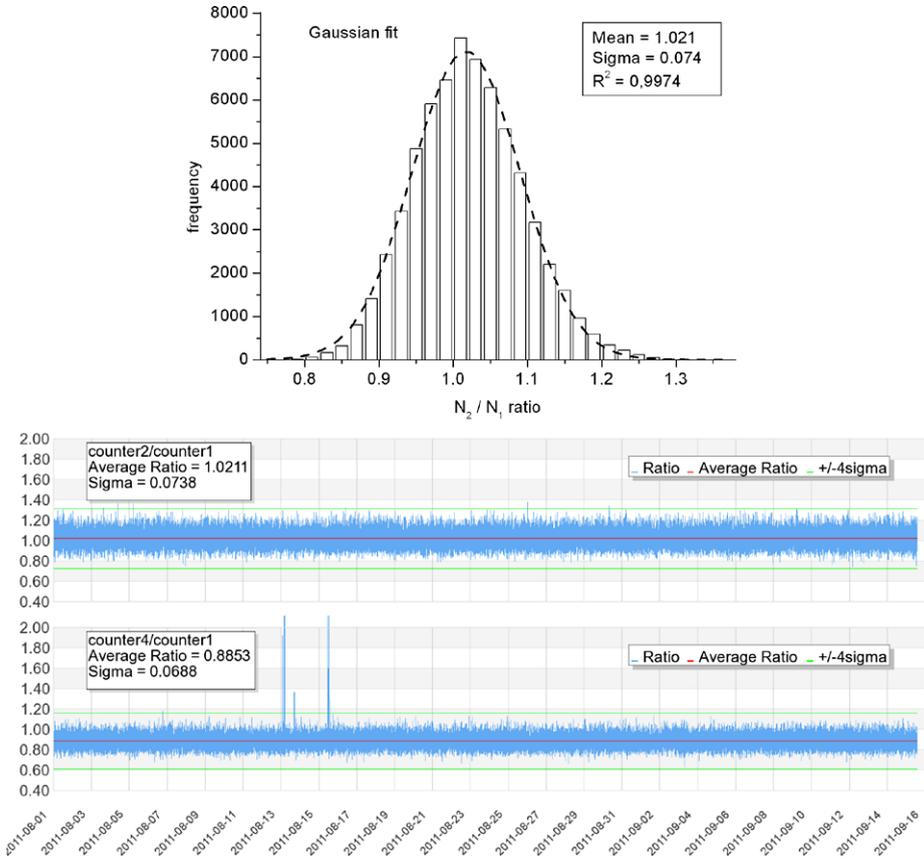
**Figure 3** The histogram of the ratio  $N_2/N_1$  (upper panel) and the time series of the ratios  $N_2/N_1$  and  $N_4/N_1$  (lower panel) based on the 1-min data of Athens station from 1 August 2011 to 15 September 2011.
