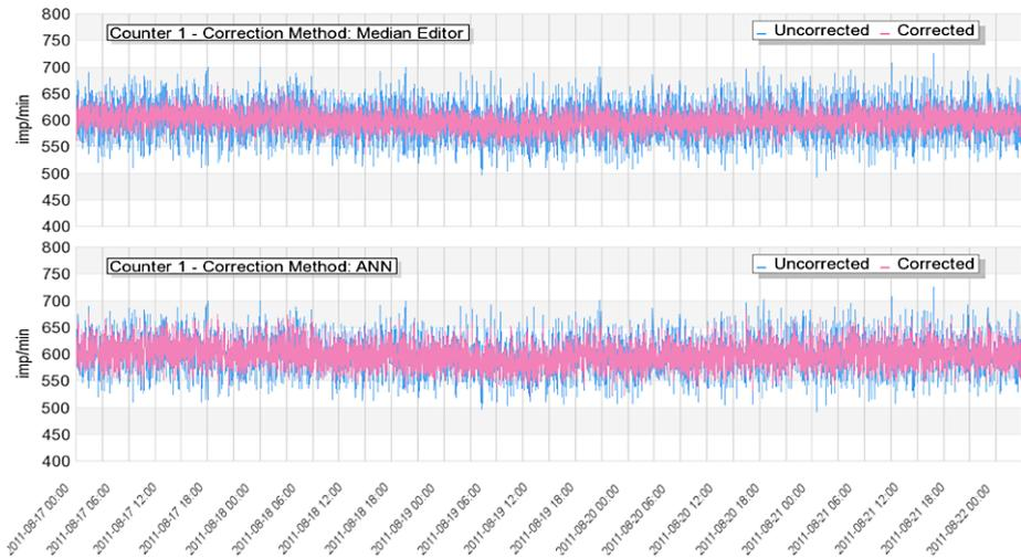
**Figure 9** Median Editor (upper plot) and ANN method (bottom plot) applied to data without errors (Athens Cosmic Ray Station for 17–21 August 2011).
