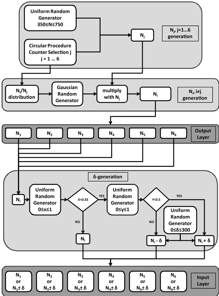
**Figure 4** Generation of training and testing samples.
