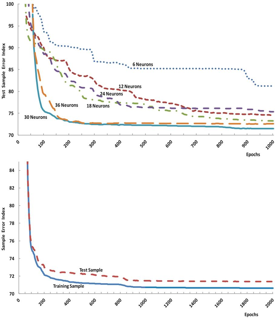
**Figure 5** The error index of the test sample for various numbers of neurons in the hidden layer (upper panel) and the error index of the training and test samples for one hidden layer with 30 neurons (lower panel).
